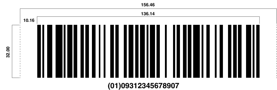
GS1-128 Barcode dimensions at nominal (100%) magnification (not to scale)
